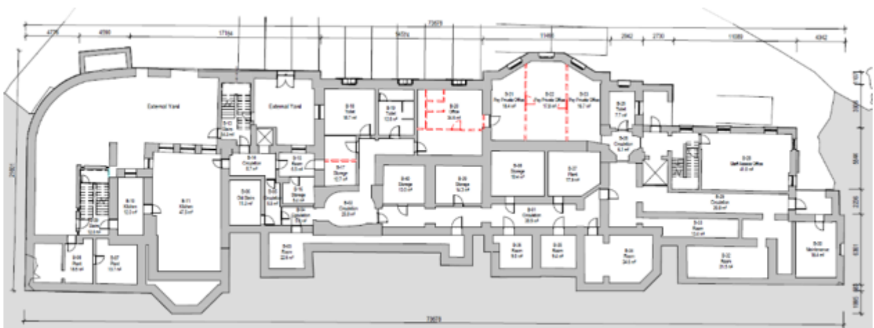
Fig.16: Basement demolition plan. Source: TOT Architects. Dashed red lines indication partitions removal.
