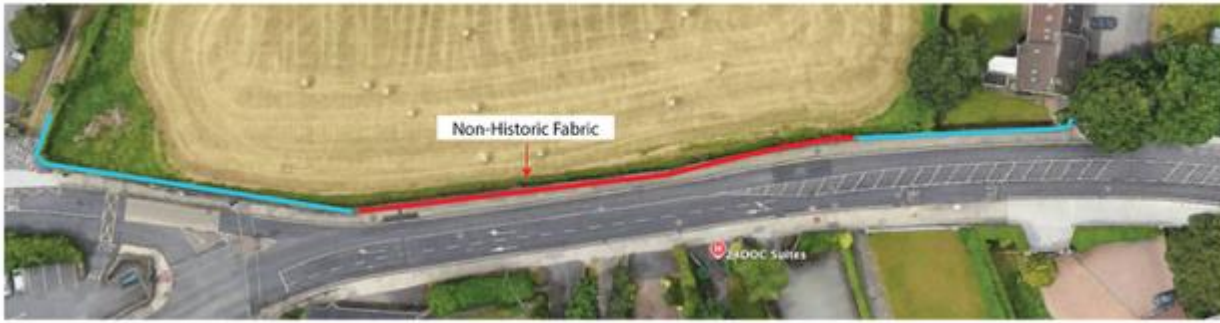
Figure 16 Indication of Non-historic Fabric of wall which has been re-built
