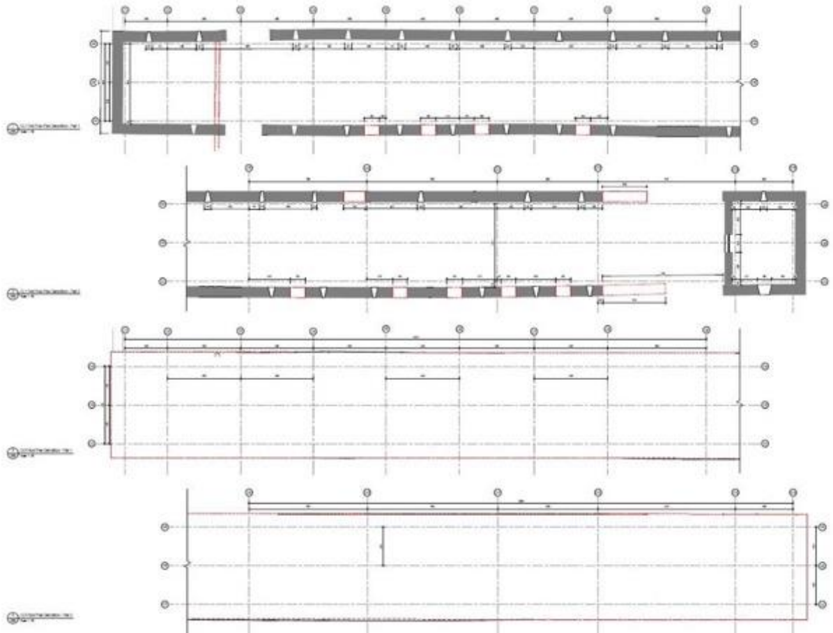
Fig.23: Demolition first floor and roof plan. From top to bottom: first floor parts 1 & 2, roof plans parts 1&2. Source: TOT Architects. Dashed red lines indication partitions removal.
