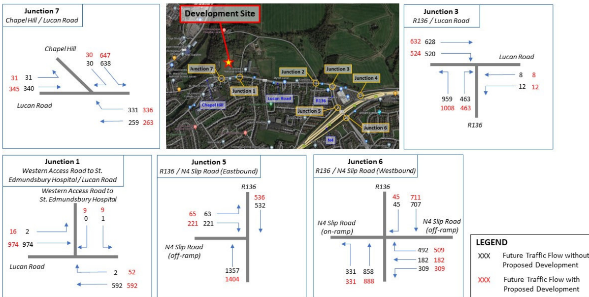
FIGURE 5.8 – 2042 DESIGN YEAR TRAFFIC FLOWS IN THE MORNING PEAK HOUR (BY USING THE TRICS DATABASE)
